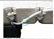
11-You can now procede to securing the air hose allong the side of the system using the provided aluminum brackets and regular "tie raps". Simply remove the lug connector, insert the aluminum bracket and reinstall the later prior to fixing the hose with the "tie raps".
